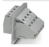
Feed-through terminal block, Connection method: Screw connection, Load current : 232 A, Cross section: 25 mm<sup>2</sup> - 95 mm<sup>2</sup>, AWG 2 - 3/0, Connection direction of the conductor to plug-in direction: 90 °, Width: 25 mm, Color: gray
