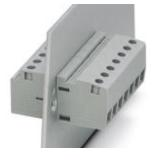
Panel feed-through terminal block, connection method: Screw connection, number of positions: 1, load current: 63 A, cross section: 0.5 mm<sup>2</sup> - 16 mm<sup>2</sup>, AWG 20 - 6, connection direction of the conductor to plug-in direction: 0 °, width: 10.1 mm, color: gray
