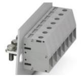
Panel feed-through terminal block, connection method: Screw connection, Cable lug connection, number of positions: 1, load current: 150 A, cross section: 16 mm<sup>2</sup> - 50 mm<sup>2</sup>, AWG 6 - 1/0, connection direction of the conductor to plug-in direction: 0 °, width: 18.8 mm, color: gray
