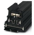
Fuse terminal block, Connection method: Screw connection, Cross section:  $0.2 \text{ mm}^2$ -  $4 \text{ mm}^2$ , AWG: 24 - 12, Nominal current: 6.3 A, Nominal voltage: 400 V, Width: 8.2 mm, Fuse type: G /  $5 \times 20$ , Fuse type: Glass, Mounting type: NS 35/7.5, NS 35/15, NS 32, Color: black
