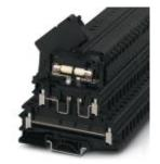
Fuse modular terminal block, Connection method: Screw connection, Cross section:  $0.2 \text{ mm}^2$ -  $4 \text{ mm}^2$ , AWG: 24 - 12, Nominal current: 6.3 A, Nominal voltage: 400 V, Width: 8.2 mm, Fuse type:  $G / 5 \times 20$ , Fuse type: Glass, Mounting type: NS 35/7.5, NS 35/15, NS 32, Color: black
