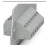
Feed-through terminal block, Connection method: Screw connection, Load current : 101 A, Cross section: 0.5 mm² - 25 mm², Connection direction of the conductor to plug-in direction: 90  $^{\circ}$ , Width: 12.1 mm, Color: gray
