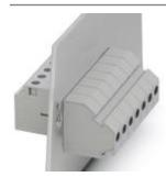
Panel feed-through terminal block, connection method: Screw connection, number of positions: 1, load current: 76 A, cross section: 0.5 mm² - 16 mm², AWG 20 - 6, connection direction of the conductor to plug-in direction: 90 °, width: 10.1 mm, color: gray
