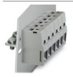
Panel feed-through terminal block, Connection method: Screw connection, Cable lug connection, Load current : 232 A, Cross section: 35 mm<sup>2</sup> - 95 mm<sup>2</sup>, AWG 4 - 2/0, Connection direction of the conductor to plug-in direction: 0 °, Width: 25 mm, Color: gray
