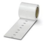
Insert label, For marking Siemens ET 200S controllers, Roll, turquoise, unlabeled, can be labeled with: THERMOMARK ROLL, THERMOMARK ROLL X1, THERMOMARK X1.2, THERMOMARK S1.1, Mounting type: snapped into marker carrier, Lettering field: 1 of 50 x 12.8 mm and 1 of 27.5 x 12.8 mm
