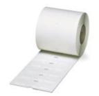
Cable marker label, Roll, white, unlabeled, can be labeled with: THERMOMARK ROLL, THERMOMARK ROLL X1, THERMOMARK X, THERMOMARK S1.1, Mounting type: Adhesive, Cable diameter: ≤46 mm, Lettering field: 25 x 38 mm
