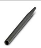
Threading pin, helps thread PMH onto the conductor; insert conductor into pin opening and slide collar on. For external conductor cross section: 3.8 - 5.4 mm
