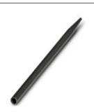
Threading pin, helps thread PMH onto the conductor; insert conductor into pin opening and slide collar on. For external conductor cross section: 2.5 - 3.3 mm
