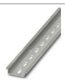
DIN rail perforated, Standard profile, width: 35 mm, height: 7.5 mm, acc. to EN 60715, material: Steel, galvanized, length: 2000 mm, Hole size: 5.2 mm x 18 mm, color: silver
