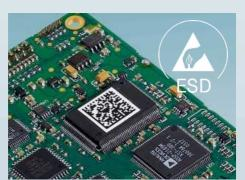
Protection against static discharge ESD-safe labels can be used to mark components and PCBs that are at risk from electrostatic discharge.
