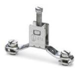
Ground modular terminal block, Connection method: Screw connection, Number of positions: 1, Cross section: 0.5 mm<sup>2</sup> - 16 mm<sup>2</sup>, AWG: 20 - 6, Width: 8 mm, Color: silver, Mounting type: NS 35/7,5, NS 35/15
