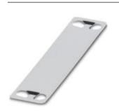
Cable marker, Stainless steel label, silver, Unlabeled, Mounting type: Assembly with cable binders, Cable diameter: 1-63 mm, Lettering field:  $23 \times 9 \text{ mm}$
