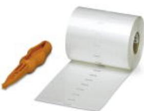
Marker for terminal blocks, Roll, white, Unlabeled, Can be labeled with: Thermomark R, Thermomark X, Thermomark S, Perforated, Mounting type: Snap into universal marker groove, Snap into flat marker groove, For terminal block width: 10.2 mm, Lettering field: 6.35 x 10.15 mm
