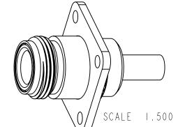
3.CRIMP FERRULE OVER BRAID AND BODY WITH AMPHENOL TOOL 277-944 AND DIE SET 227-1221-57, CAVITY 'A' .HEX CRIMP SIZE .213"
