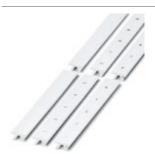
Zack marker strip, Strip, white, Unlabeled, Can be labeled with: Plotter, Mounting type: Snap into tall marker groove, For terminal block width: 16.3 mm, Lettering field: 10.5 x 16.25 mm
