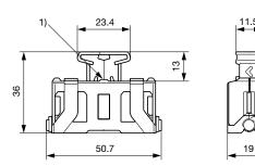
Position for optional terminal marking (terminal block width: 5.2 mm, lettering field: 4.6x5.1 mm, e.g. item 0818153 from Phoenix Contact) 50.7 mm
