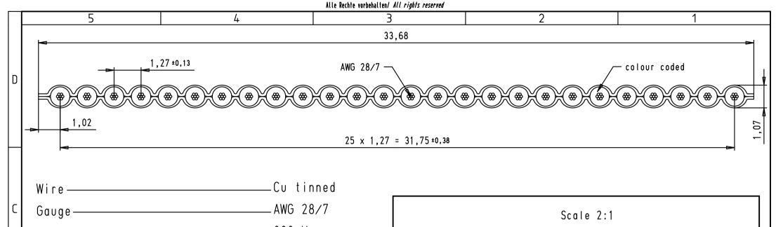
Voltage rating————300 Vr.m.s Conductor resistance — 221 m $\Omega$ /m Capacity unbalanced———49 pF/m Impedance unbalanced———105  $\Omega$ Signal delay——5,2 ns/m Insulation material —————PVC Flammability rating——UL: VW1 Insulation resistance — 1000  $M\Omega/km$
