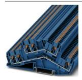
Double-level terminal block, Cross section: 0.14 mm<sup>2</sup> - 4 mm<sup>2</sup>, AWG: 26 - 12, Connection type: Push-in connection, Width: 5.2 mm, Color: blue, Mounting type: NS 35/7,5, NS 35/15
