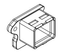
Connector pitch on panel: Axis X = 27 mm and Axis Y = 21 mm Receptacle mating side according to 600076-3-106 IEC - variant 04
