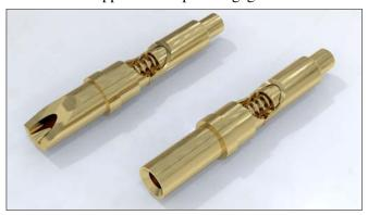
Plated with  $20\mu$ " of gold over nickel on each precision-machined component and  $10\mu$ " of gold over nickel on the beryllium copper spring, the 0962 is as durable as it is multi-faceted.
