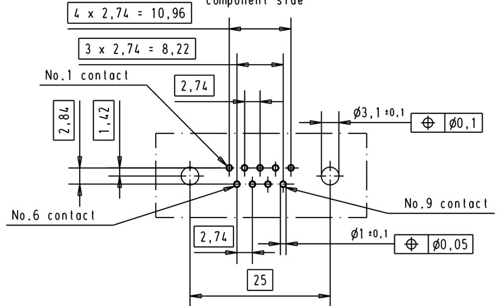
Connector retention and insertion forces on the PCB = 25 / 80 newtons
