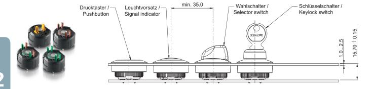
For printed circuit board hole patterns, see RAFIX 22 FS-Technology contact blocks
