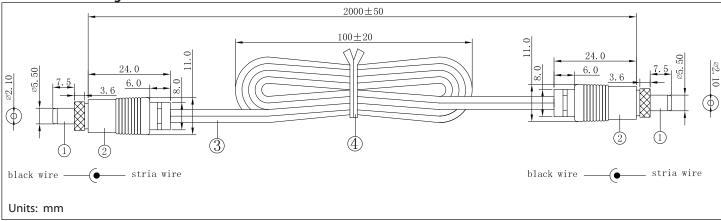
**tolerance** X: ±0.5 mm .X: ±0.3 mm .XX: ±0.05 mm applicable unless otherwise indicated in specification or on drawings Tensility International Corporation reserves the right to substitute parts which are functionally equivalent to the ones specified.
