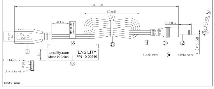
tolerance X: ±0.5 mm .X: ±0.3 mm .XX: ±0.05 mm applicable unless otherwise indicated in specification or on drawings Tensility International Corporation reserves the right to substitute
