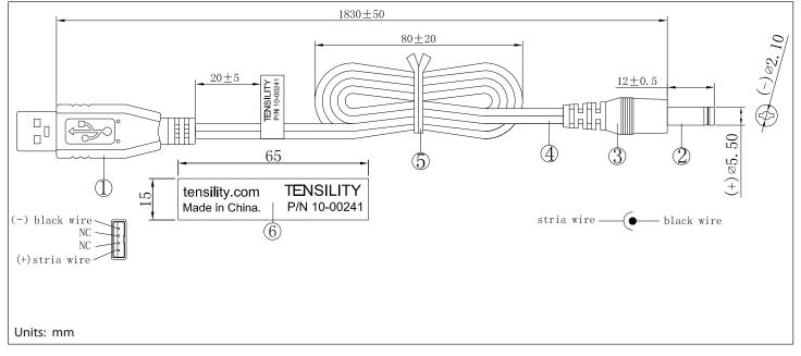
tolerance X: ±0.5 mm .X: ±0.3 mm .XX: ±0.05 mm applicable unless otherwise indicated in specification or on drawings Tensility International Corporation reserves the right to substitute parts which are functionally equivalent to the ones specified.
