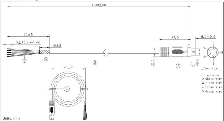
**tolerance** X: ±0.5 mm .X: ±0.3 mm .XX: ±0.05 mm applicable unless otherwise indicated in specification or on drawings Tensility International Corporation reserves the right to substitute parts which are functionally equivalent to the ones specified.
