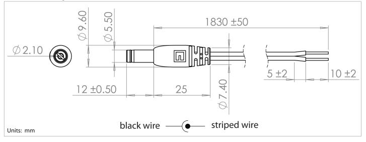
**tolerance X: ±0.5 mm .X: ±0.3 mm .XX: ±0.05 mm** applicable unless otherwise indicated in specification or on drawings Tensility International Corporation reserves the right to substitute
