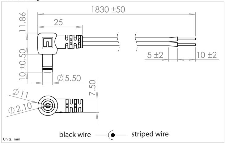
**tolerance X: ±0.5 mm .X: ±0.3 mm .XX: ±0.05 mm** applicable unless otherwise indicated in specification or on drawings Tensility International Corporation reserves the right to substitute parts which are functionally equivalent to the ones specified.
