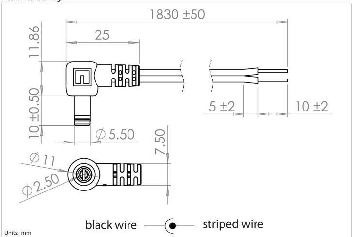
**tolerance** X: ±0.5 mm .X: ±0.3 mm .XX: ±0.05 mm applicable unless otherwise indicated in specification or on drawings Tensility International Corporation reserves the right to substitute parts which are functionally equivalent to the ones specified.
