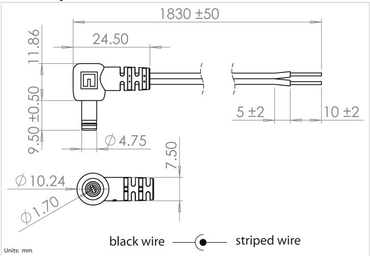
**tolerance** X: ±0.5 mm .X: ±0.3 mm .XX: ±0.05 mm applicable unless otherwise indicated in specification or on drawings Tensility International Corporation reserves the right to substitute parts which are functionally equivalent to the ones specified.
