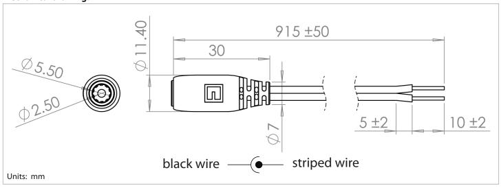
**tolerance** X: ±0.5 mm .X: ±0.3 mm .XX: ±0.05 mm applicable unless otherwise indicated in specification or on drawings Tensility International Corporation reserves the right to substitute parts which are functionally equivalent to the ones specified.
