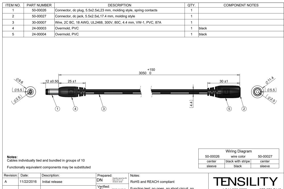
Function test: no open, no short circuit, no Digitally signed by GL Date: 2016.11.22 13:41:22 -08'00' 800 877.670.7118 GL tel 1.541.323.3228 intermittent fax 1.541.323.4202 web tensility.com Dimensions are in millimeters. Size: Part number: Description: Tolerances: Cable, 3050 mm, 5.5x2.5x12 mm 50-00026 dc 10-02397 А ± 0.5 mm X: plug to 5.5x2.5 mm 50-00027 dc jack, 18 AWG, X.X: ± 0.3 mm  $(\bigcirc)$ Scale: 1:1 Sheet 1 of 1 30-00007 wire X.XX: ± 0.05 mm  $\mathbf{2}$ 1
