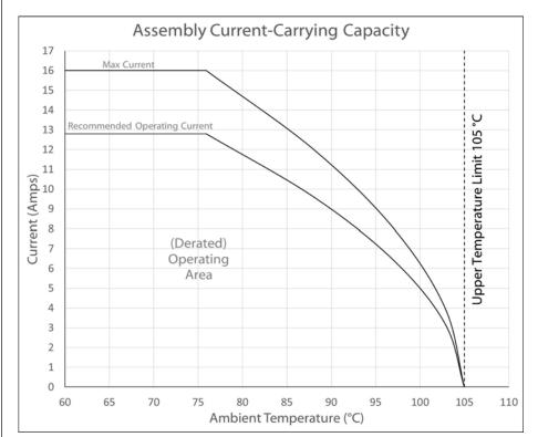
Testing based on IEC 60512-5-2. Max current curve generated with isolated test article under controlled environmental conditions,  $and does \ not \ take \ into \ account \ external \ factors \ such \ as \ housings \ or \ circuitry. \ Recommended \ operating \ current \ curve \ (derated \ to \ operation \ derated \ to \ operation \ derated \ to \ operation \ derated \ derat$ 80% of max values) accounts for external factors, manufacturing variation, and error in temperature measurements.
