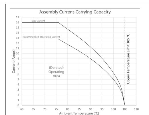
Testing based on IEC 60512-5-2. Max current curve generated with isolated test article under controlled environmental conditions, and does not take into account external factors such as housings or circuitry. Recommended operating current curve (derated to 80% of max values) accounts for external factors, manufacturing variation, and error in temperature measurements.
