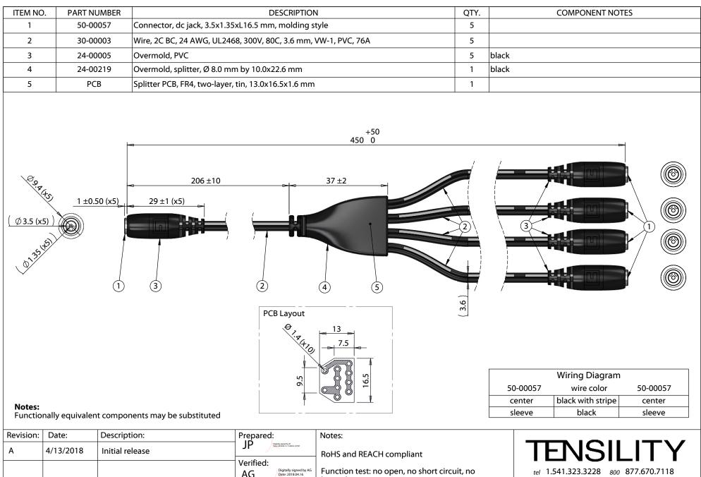
Digitally signed by AG Date: 2018.04.16 16:54:44 -07'00' AG intermittent fax 1.541.323.4202 web tensility.com Dimensions are in millimeters. Part number: Description: Size: Tolerances: Cable, 450 mm, 3.5x1.35 mm 50-00057 dc jack to y-А 10-02760 ± 0.5 mm Х: split to 4x 3.5x1.35 mm dc jack, 24 AWG X.X: ± 0.3 mm Sheet 1 of 1 Scale: 1:1 X.XX: ± 0.05 mm 3 2
