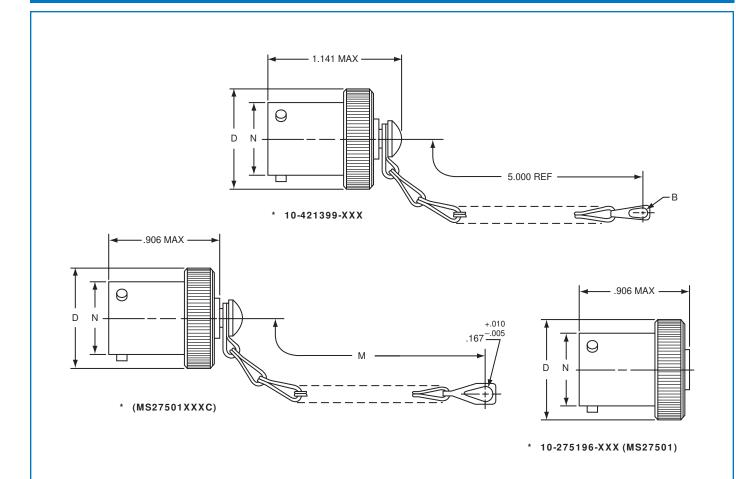
\* To complete order number, add shell size and suffix number. For example, shell size 11 with cadmium plate, nickel base would be 10-421399-117, MS27501A11C or MS20048A11.
