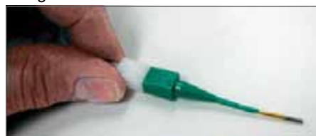
Plastic tool with contact in proper position.
