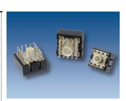
The RADSOK® PowerBlok™'s compact footprint  $\frac{1}{2}$ " x  $\frac{1}{2}$ " can supply up to 70A to backplane power connections. Current is distributed over 16 compliant pins. The PowerBlok™ is available for top or bottom entry and offered with a touch-proof cover.
