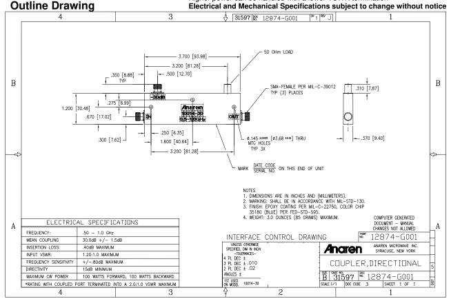
**NOTES**: The power rating applies when coupled port VSWR is 2.0:1 or less. Higher power can be handled with a lower VSWR termination **Electrical and Mechanical Specifications subject to change without notice**
