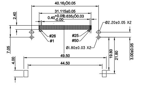
7. THE HOUSING WILL WITHSTAND EXPOSURE TO 260°C PEAK TEMPERATURE FOR 10 SECONDS IN A CONVECTION, IR OR VAPER PHASE REFLOW OVEN. 8. THIS PRODUCT (10053867-XXXXLF) MEETS THE EUROPEAN UNION DIRECTIVE AS DESCRIBED IN GS-22-008.
