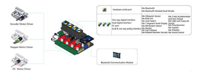
Wireless communication interface – for adding Bluetooth module or 2.4G module (require corresponding communication module)
