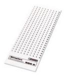
Marker cards, Card, white, Labeled, Printed horizontally: Consecutive numbers: Front 1 - 250, back 251 - 500, Mounting type: Snap into tall marker groove, Snap into flat marker groove, For terminal block width: 6.2 mm, Lettering field: 6 x 6.1 mm
