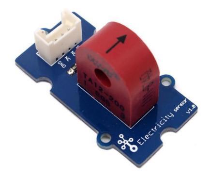
The Electricity sensor module is a member of Grove. It is based on the TA12-200 current transformer which can transform the large AC into small amplitude. You can use it to test large alternating current up to 5A.
