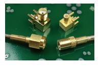
SMB connectors are 30% smaller than SMA connectors.
