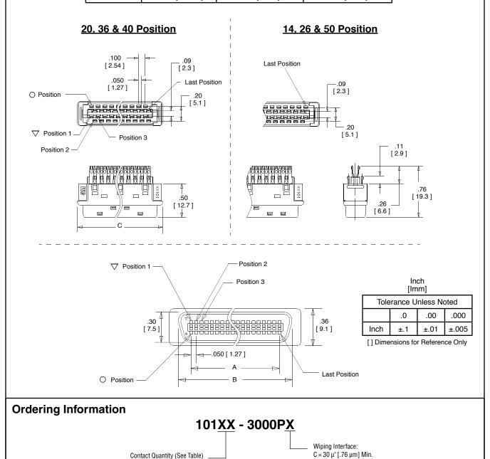
Note: This solder plug connector must be used with only 3M Non-Shielded Shell Kits 103XX-52F0-008 Series and 103XX-52A0-008 Series.
