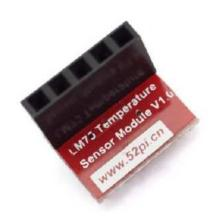
Temperature sensor for Raspberry Pi -LM75
